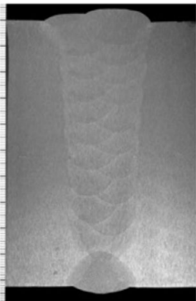
100 mm cross section (avg. steel thickness), Monopile: 2200 MT weight / 99 M long Photo courtesy of The Lincoln Electric Company
